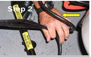
Leaving at least a 12" loop of chemical hose between your hand and the valves on the bottom of the cylinders, grasp both hoses in one hand and pull the hoses underneath the lower front frame.
