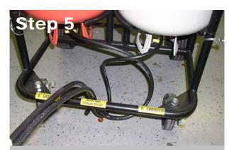
Remember to leave at least a 12" loop of chemical hose between the STRAIN RELIEF fixture and the valves on the bottom of the chemical cylinders.
