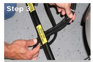
Loop both chemical hoses back through the STRAIN RELIEF fixture near the bottom of the chemical cylinders. Position the chemical hoses back over the top of the lower front frame.
