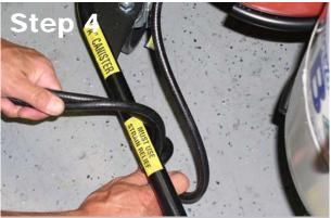
Gently tug on the chemical hoses to ensure the STRAIN RELIEF fixture is properly engaged. If properly engaged, the yellow valves on the bottom of the cylinders will not be pulled when the chemical hoses are pulled.
