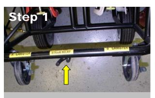
Locate the STRAIN RELIEF fixture underneath the lower front frame of the unit. It is "U" shaped and lies directly underneath the label "MUST USE STRAIN RELIEF."
