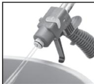
4. Lubricate o-ring with lubricant (provided). Attach spray nozzle – align slots with notch on gun, push and twist clockwise to lock in place. Foam should be off-white in color (not white or dark brown – for more information see Troubleshooting section). Carry unit by handle attached to tanks – never lift or pull by hoses.
