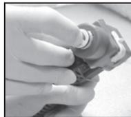
During nozzle changeover, clean and lubricate o-ring and remove any buildup from orifices in gun barrel. **Note: To help product performance in cold spraying environments, you may carefully spray foam inside carton to help maintain the temperature of chemicals in tanks.**
